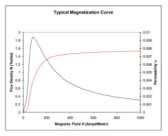
density in the respective material. The preference for magnetic flux to travel through a ferromagnetic material is not constant but changes with the strength of the magnetic field.
