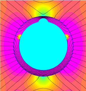
Comparing the flux density near the surface of the tubing near the wear and opposite the wear we see the effect with an amplitude of around 2.5 mT or about 25 guass in this simulation. This is well within the capabilities of a standard linear Hall Effect sensor.
