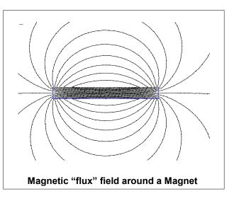
flux density. A common simple experiment to visualize a magnetic field is the use of iron filings (a magnetic material), sprinkled over a sheet paper (non-magentic material) covering a magnet.
