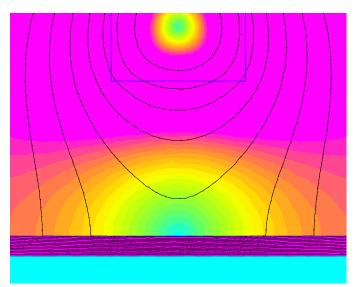
The first diagram shows the normal flux lines and color encoded flux density with no defects.
