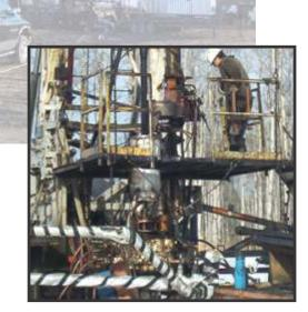
Tubing can be tripped through the ScanNex® scanner either coming out of the well or on the way in the well.
