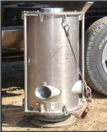
The heart of our service is the ScanNex® scanner. Based on magnetic flux leakage and flux deviation/redistribution principles with microprocessor controlled solid state sensor arrays, these units provide highly reliable and repeatable quality inspections. We, at RD Scan Inc., own and operate this exclusive technology.
