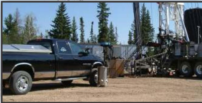
Magnetic flux leakage and deviation/redistribution caused by anomalies in the tubing are detected by the sensor arrays. The sensor information is sent to a computer in the truck where the data is analyzed, graphed, interpreted and stored. The ScanNex® patented technology
